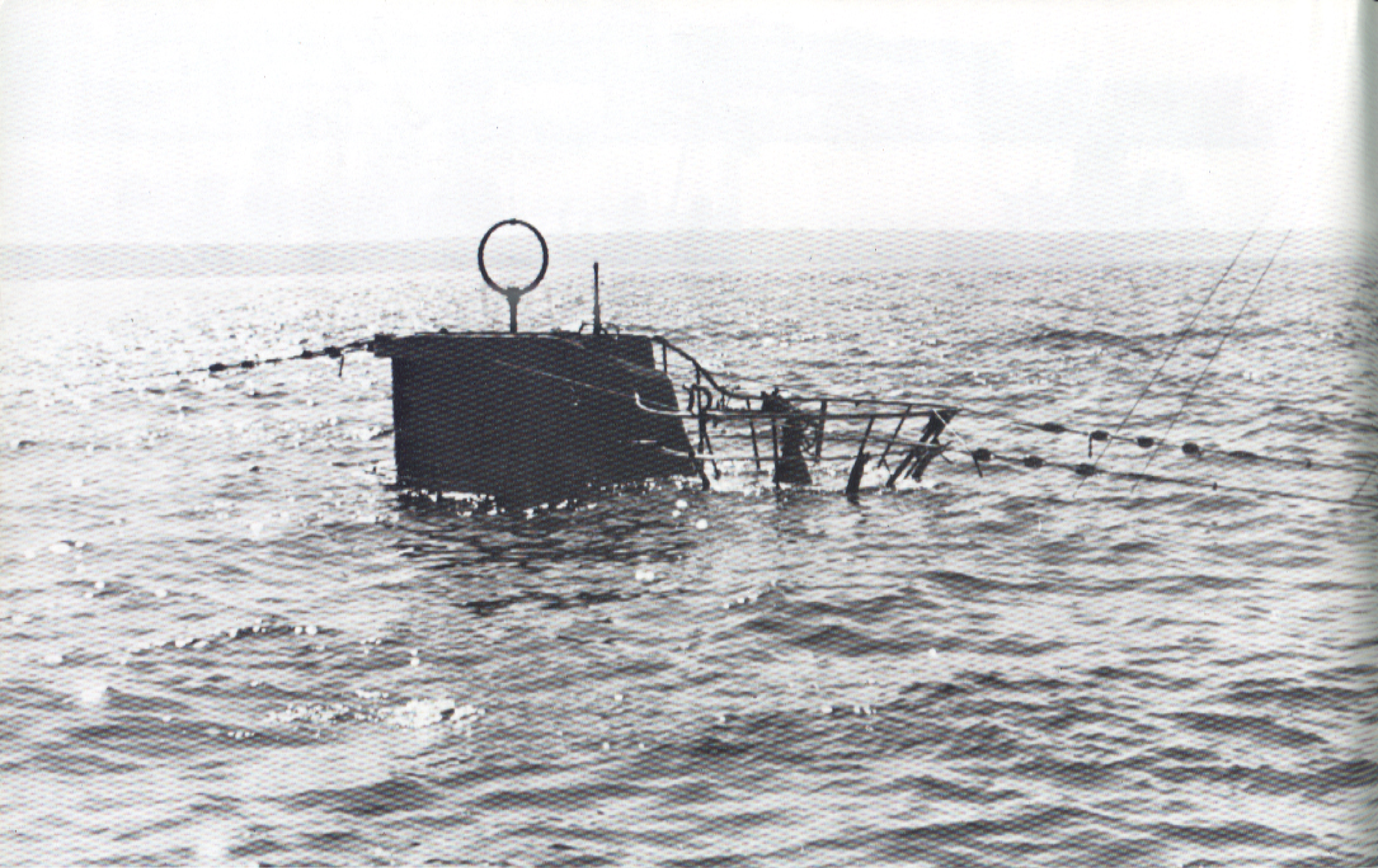
U-86 (Type VII B) on a practice run in the Baltic Sea. The boat is being taken to diving depth when not in motion as a test. The Type VII boats could disappear from the surface in thirty seconds.
